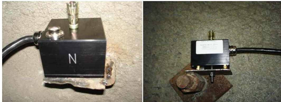
Figure 3 Surface Sensors mounted on 12m long rock bolts
