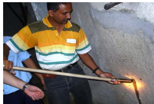
Figure 2 Borehole geophone with installation tool
